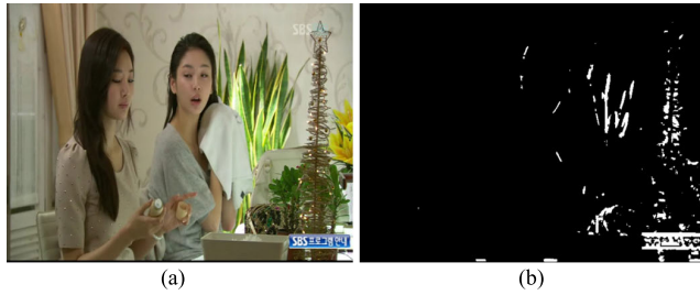
FIGURE 4. Generation of the text map using directional coherence values: (a) original image and (b) text edge map (Black pixels denote non-text regions and white pixels denote text regions). ©Secret Garden SBS.
