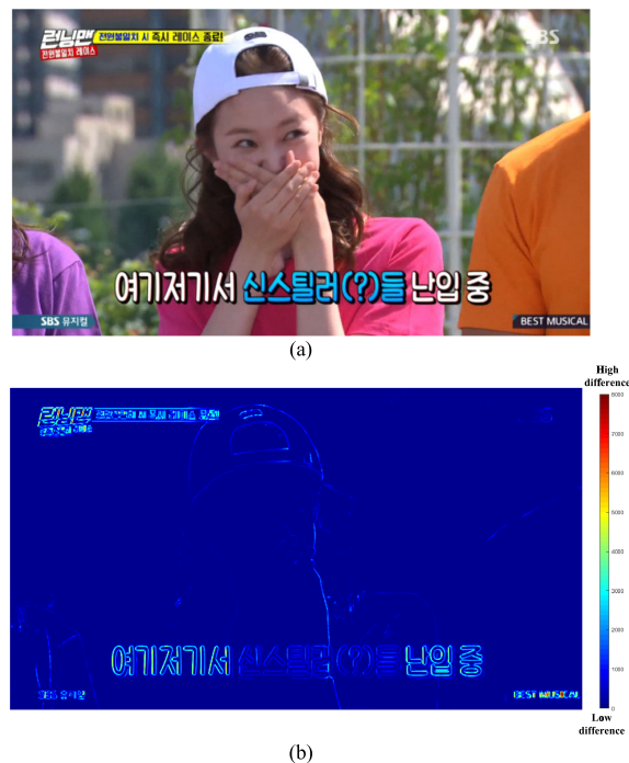
FIGURE 3. Directional coherence values obtained from original image: (a) original image and (b) directional coherence values for each pixel (Note that directional coherence value of the scrolling-text or text region is much larger than that of flat and highly-textured regions). ©Running Man SBS.
