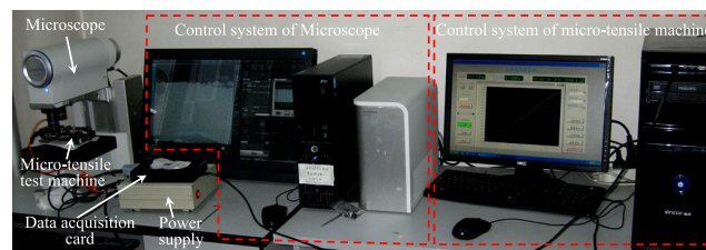
FIGURE 14. Experimental set up for micro-tensile test.
