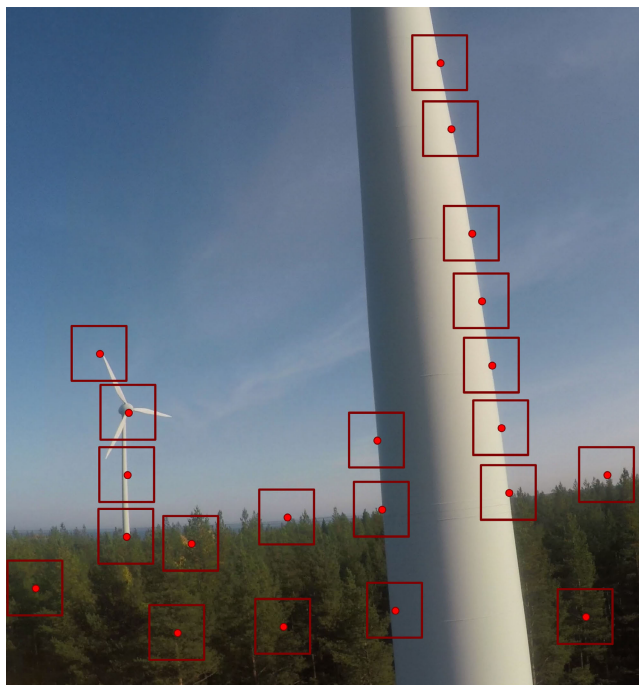
FIGURE 3. A sample of features detected on the wind turbine tower and the surrounding environment.
