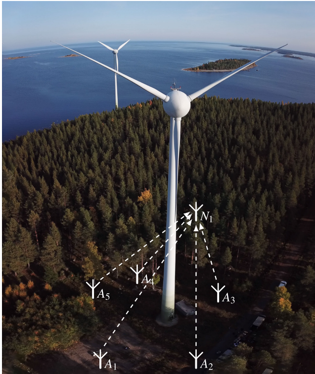
FIGURE 7. An overview of the UWB localization system, where A_1 - A_5 are the stationary anchors and N_1 is the tracked node mounted on the MAV, while the dashed lines highlight the measured distances.
