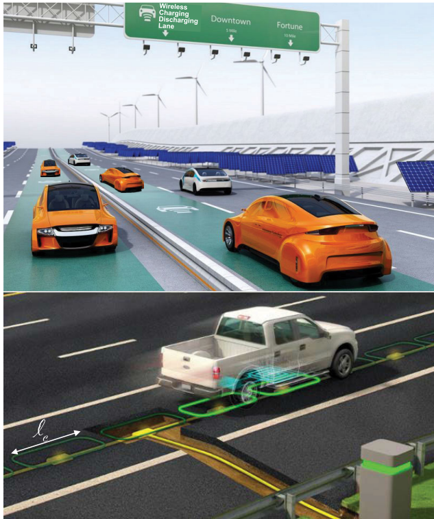
FIGURE 1. Illustration for EVs charged/discharged by wireless charging-discharging lanes with renewables along roadsides (upper), and under-road wireless charging-discharging segments (lower). (Photos are adopted with modifications from https://www.magment.de/de-dynamic-wireless-charging , and https://en.reset.org/blog/turning-roads-smart-charging-solutions-electric-cars-07052018 ).
