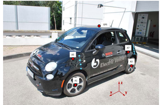
FIGURE 1. Fiat 500e test car. Sensor positions A1, A3 (wheel carrier), A5 (dome bearing), A7 (top of shock absorber).
