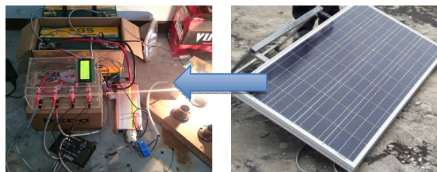
FIGURE 6. Developed monitoring system to collect data from PV system.
