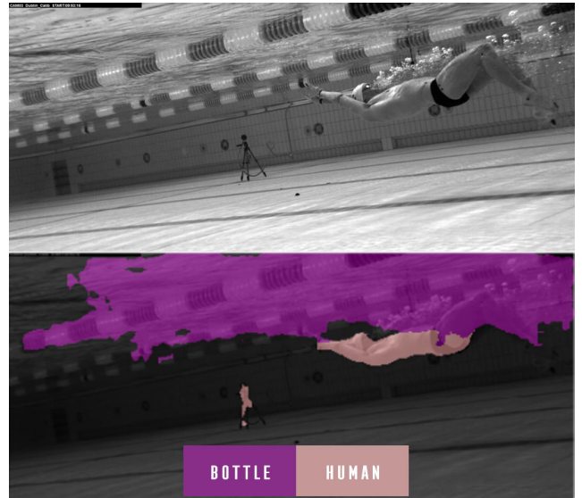
FIGURE 2. Top: original image. Bottom: silhouette extracted using DeepLabv3+ (trained on PASCAL VOC).
