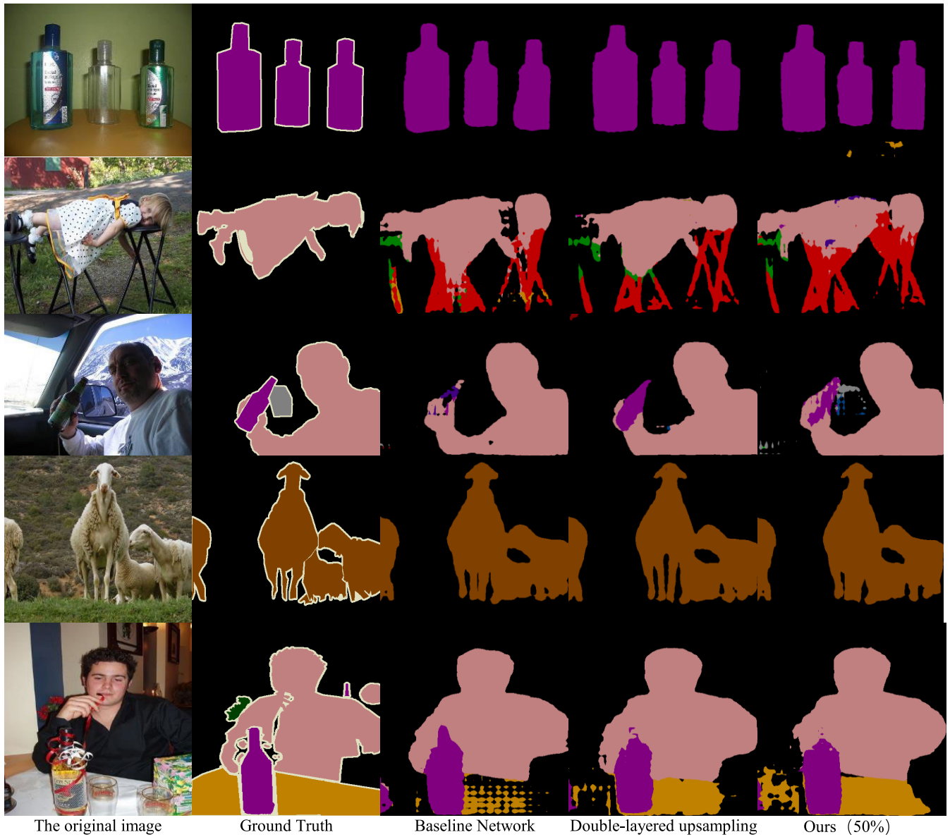
FIGURE 6. The results of the segmentation prediction using a fully-supervised baseline network, a double-layered upsampling network and the proposed algorithm with 50% of the samples.
