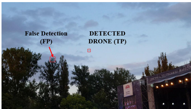
FIGURE 19. Best Haar Cascade model detection with a true positive detection on a small-sized (measured as a percentage of overall image) drone at an incurred cost of false detection.
