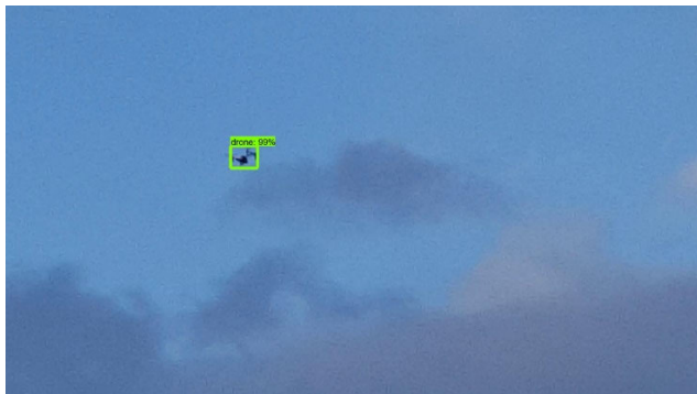
FIGURE 24. ANN detection model (as obtained for iteration=867503) deployed over a drone footage. The model was shown to be very effective in detecting model presented in the figure but often failed to detect drones of a small size (calculated as a percentage of overall image).
