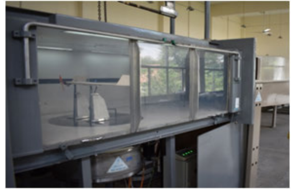
(a) FWMAV installed inside test section of subsonic wind tunnel. Rectangular test section of 2\text{ ft} \times 3\text{ ft} \times 6\text{ ft} and six strain gauge pyramidal balance is shown.
