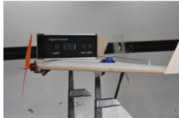
(b) FWMAV at angle of attack of 2^\circ with Gemfan 5030 propeller blade. Wind tunnel tests were conducted for varying advance ratios with current attitude.
