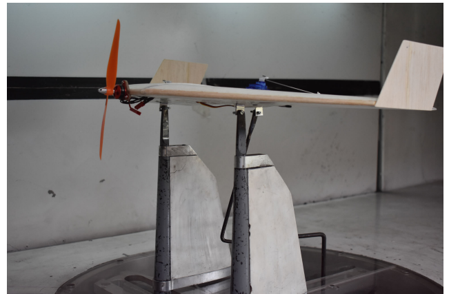
FIGURE 9. Support System inside Wind Tunnel Test Section. The support system is used to position test objects at correct attitude for conduct of wind tunnel tests. Tare and Interference drag generated by these supporting structure is estimated and removed from overall drag of the object using equations 3 to 7.
