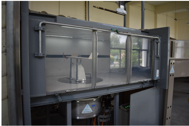
FIGURE 8. Wind Tunnel used for Wind Tunnel Testing of FWMAV. The figure shows test section of wind tunnel and six strain gauge complete pyramidal balance system. FWMAV is installed inside test section.
