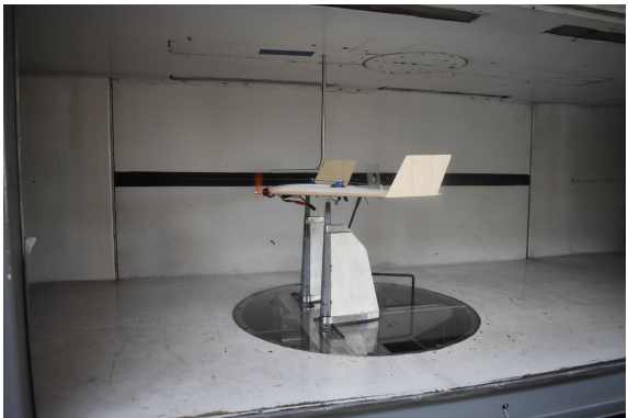
(c) Wind tunnel testing with pitot-static probe installed at 75% of blade radius. Propeller induce velocity was recorded as 0.2011 \frac{m}{s} for wind tunnel test ID T9.
