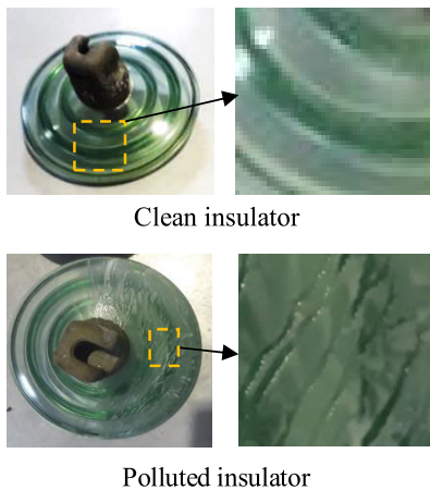
FIGURE 3. Clean and polluted glass insulator.
