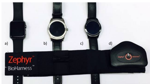
FIGURE 1. Three different COTS smartwatches and the ground truth device used for heart rate measurements: (a) Apple Watch, (b) LG Urbane, and (c) Samsung Gear S2 and (d) Zephyr BioHarness chest strap for ground truth measurements.
