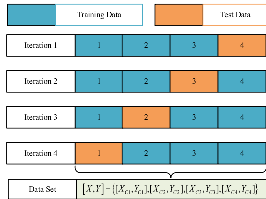
FIGURE 12. The schematic of leave-one-out cross validation process.
