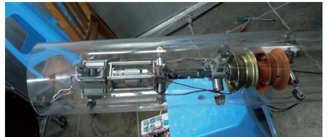
FIGURE 23. Photographs of the robot climbing the inclined pipe.
