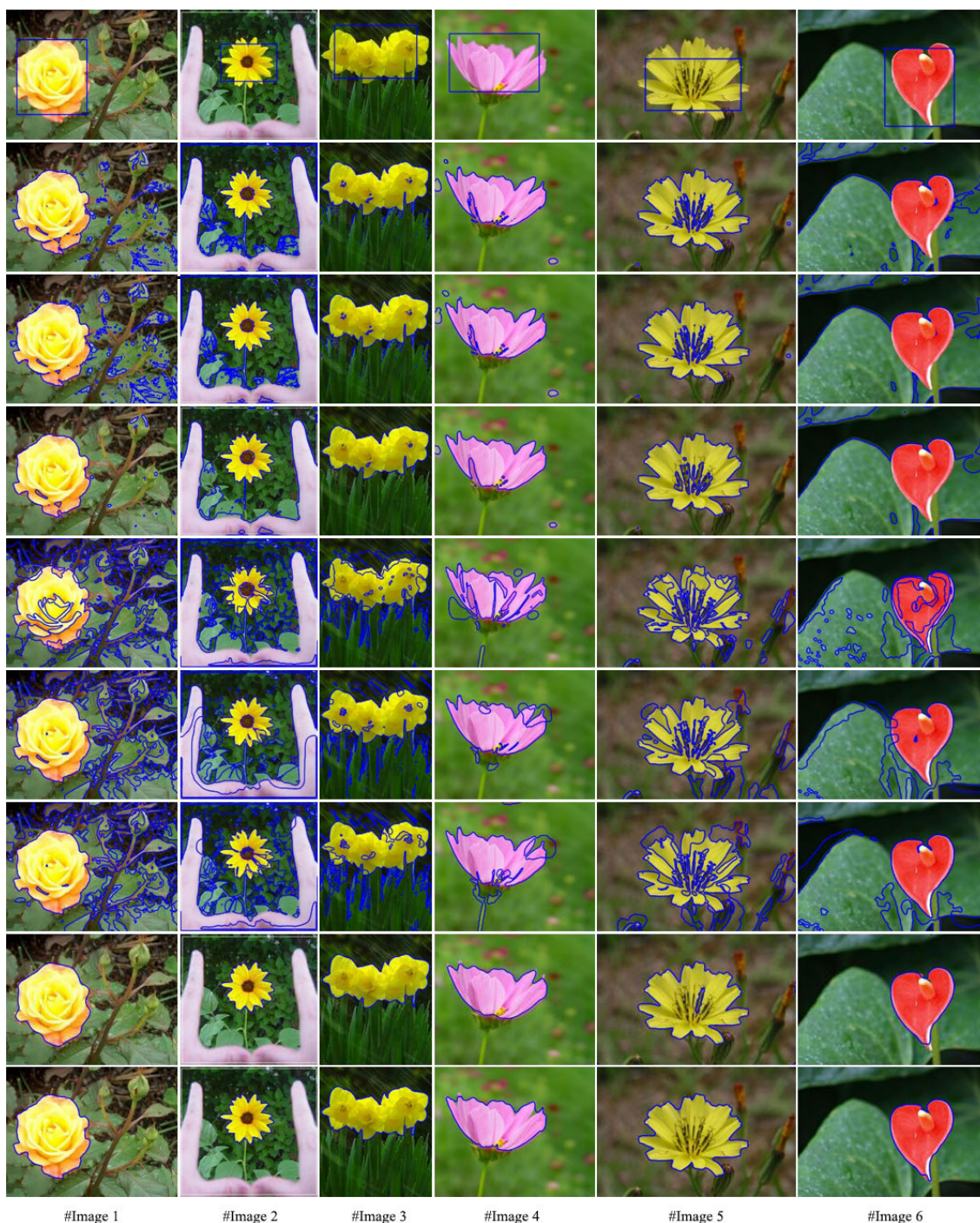
FIGURE 12. The final stopping positions of the zero level set for natural image from MSRA-B database using different models. Row 1: The original images with initial contours marked by blue line. Rows 2-9: Results of CV, FEBAC, FRAGL, EWF, LBF, LIF, GLSEPF and our model.
