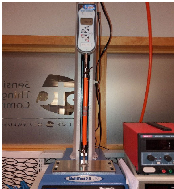
FIGURE 22. OFEF joint sample for test on Mecmesin MultiTest 2.5-Dv.
