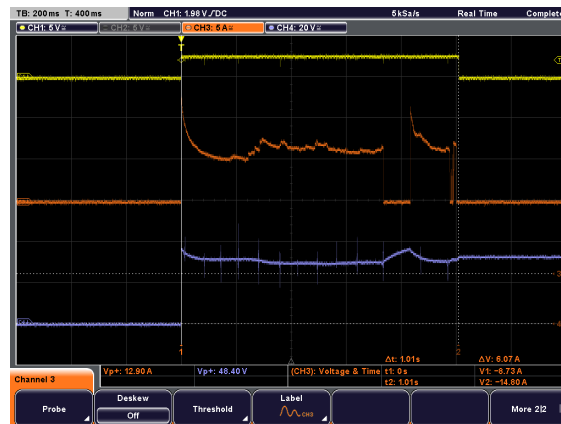
FIGURE 24. OFEF joint voltage and current spikes, as well as fusing with an 80% duty cycle.
