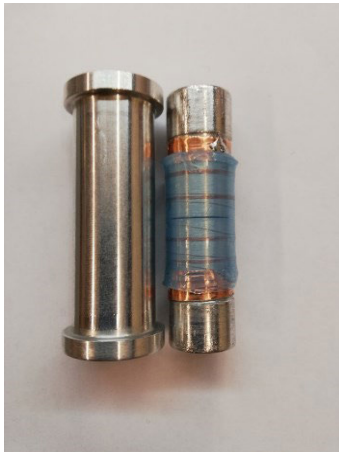
FIGURE 14. Fabricated optical fiber microduct electrofusion joint with mold.
