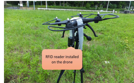
FIGURE 9. Experimental environment. (a) Experimental setup. (b) RFID reader installed on the drone.
