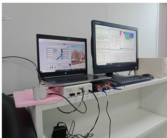
FIGURE 5. Experimental setup for logging the single constellation and multi-constellation GNSS data at the observation sites.
