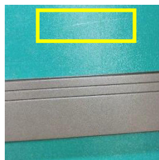
FIGURE 13. Flawless sample with abrasion mark defect in background area.
