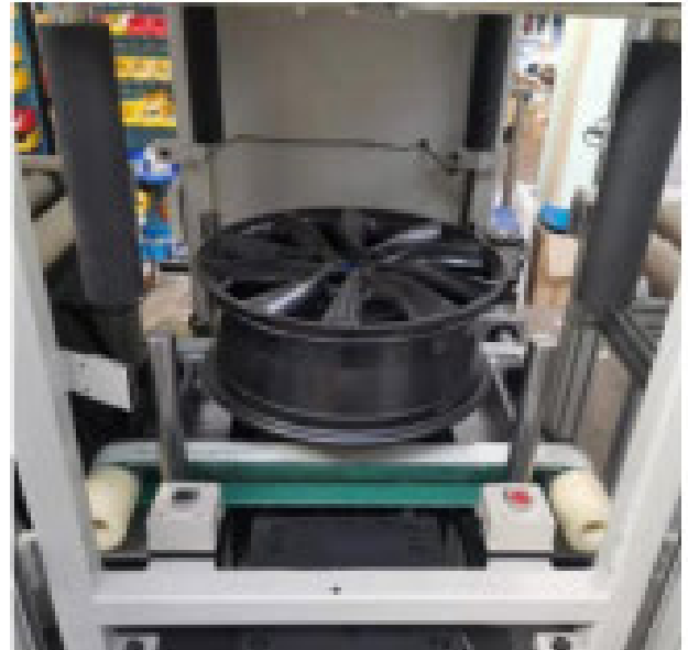
FIGURE 2. Spindle of the wheel dynamic balancing machine.
