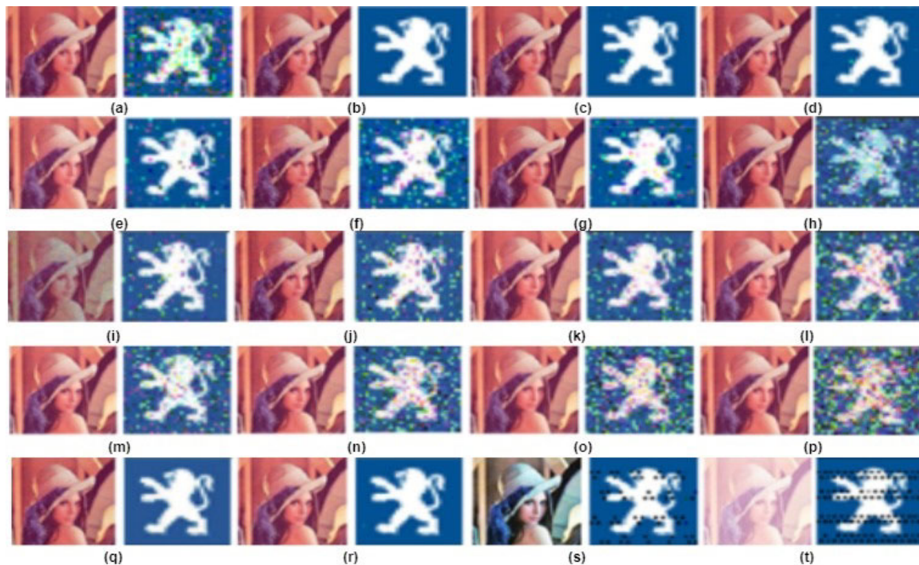
FIGURE 12. The watermarked image (Lena) and extracted watermark (Peugeot logo) after applying non-geometric attacks (a) JPG (30), (b) JPG (90), (c) JPG 2000 (5:1), (d) JPG 2000 (10:1), (e) S&NP (2%), (f) S&NP (10%), (g) GN (1%), (h) GN (3%), (i) SN (2%), (j) PN, (k) LPF (100,1), (l) LPF (100,3), (m) MF (2×2), (n) MF(3×3), (o) WF (3×3), (p) WF(5×5), (q) SH (2%), (r) BL (2%), (s) HE, (t) GC.
