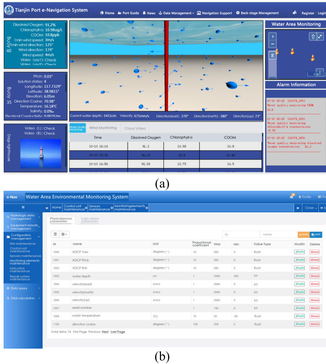
FIGURE 9. Shore-based environmental monitoring system. (a)Real-time monitoring information and data management module; (b) Comprehensive configuration module.
