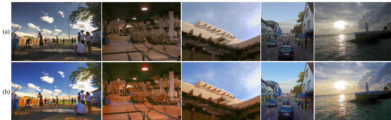
FIGURE 4. Enhanced images of low-light images shown in Fig. 3 (a) by (7): (a) mapping RGB channels; (b) mapping the value component in HSV space.
