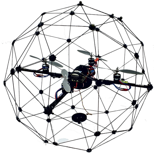
FIGURE 2. Quanser QBall 2 quadrotor.
