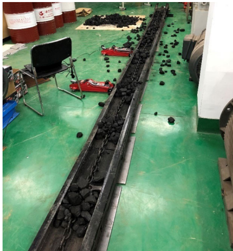
FIGURE 7. Loaded condition of the scraper conveyor test bench.
