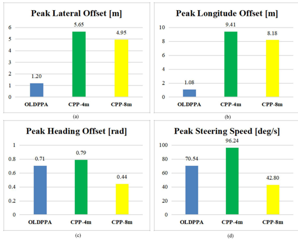
FIGURE 14. Comparison of experiment results with OLDPPA, CPP-4m, and CPP-8m for the parabolic path. (a) Peak lateral offset, (b) Peak longitude offset, (c) Peak heading offset, (d) Peak steering speed.
