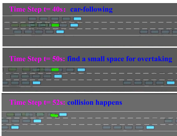
FIGURE 13. Another representative testing driving condition: the ego vehicle make a dangerous lane changing and a collision happens.
