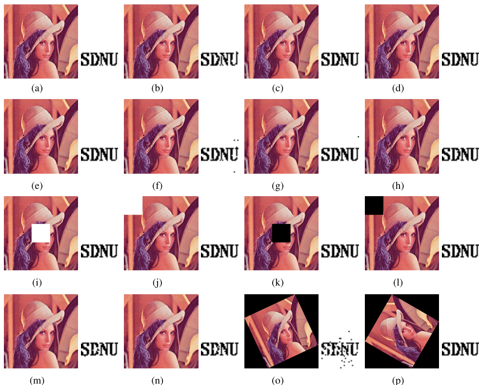
FIGURE 7. Results under different types of attacks and recovered watermark from Lena image (a) Gaussian Noise (var = 0.002) (b) Gaussian Noise (var = 0.003) (c) Salt&Pepper noise (density = 0.002) (d) Salt&Pepper noise (density = 0.003) (e) JPEG with QF = 30 (f) JPEG with QF = 50 and Gaussian noise (0.002) (g) Gaussian filter (3, 3) (h) Median filter (3, 3) (i) Centred Cropping 1/16 (128 × 128 by white) (j) Left upper cropping 1/16 (128 × 128 by white) (k) Centred Cropping 1/16 (128 × 128 by black) (l) Left upper cropping 1/16 (128 × 128 by black) (m) Scaling 0.25 (n) Scaling 0.33 (o) Image rotation (angle = 25°) (p) Image rotation (angle = 60°).
