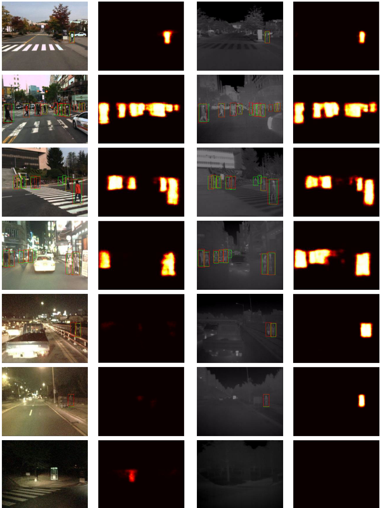
FIGURE 9. Examples of the learned attention maps of the spatial-wise weighting mechanism. The 1 to 3 and 4 to 7 rows show daytime and nighttime scenes respectively. The first and the third column show the visible and thermal input respectively, the second and the fourth column show their saliency predictions respectively generated by the PiCANets embedded in the backbones. Note that the red and the green bounding boxes (BBs) represent the BB prediction and BB ground truth, and the dark green boxes with thinner line represent the ignored BB ground truth.
