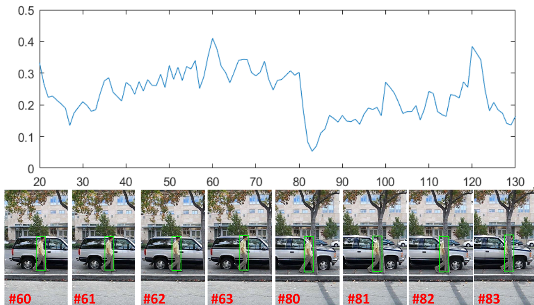
FIGURE 3. Confidence scores and visualization of selected tracking results. The fluctuation in reliability of frames 60-63 is caused by background changes. The sudden change in the reliability of frames 80-83 is caused by the occlusion of the object.
