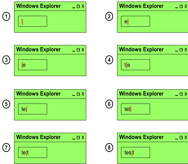
Figure 9. Inserting the text test into WE’s input box based on a random character insertion order with a corresponding movement of the caret position. The caret position is highlighted red.
