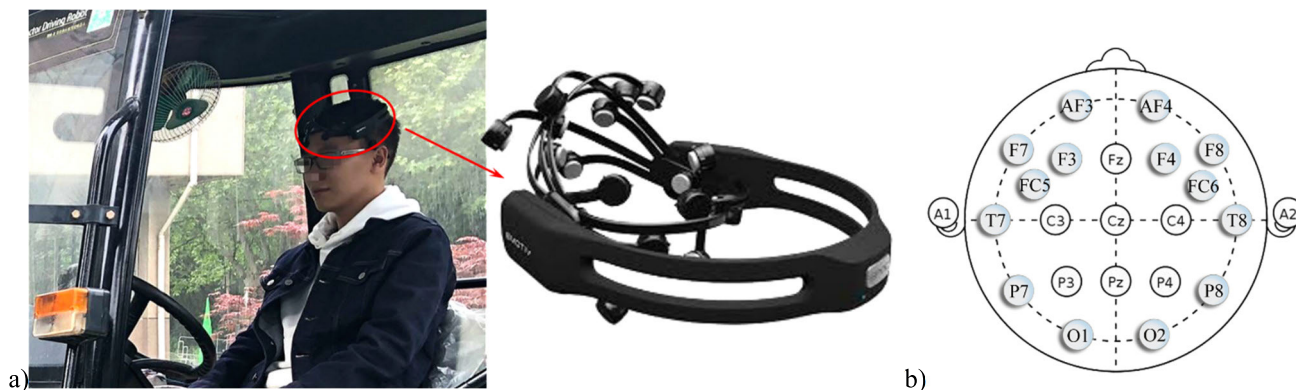
FIGURE 1. Emotiv EPOC+ and electrode setting. a) the Emotiv-EPOC+ system. b) 10/20 electrode placement system.
