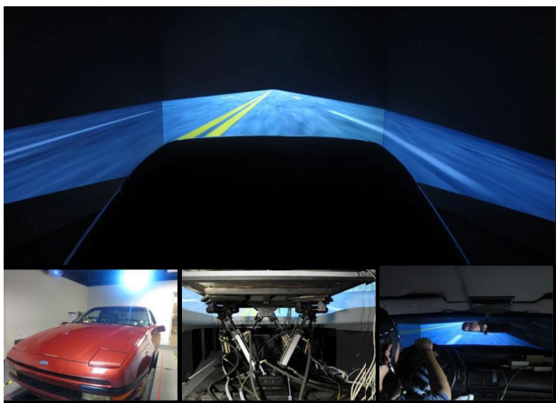
FIGURE 4. Depicting the experimental setup that was used during the acquisition of the drivers' responses during the simulated driving experience. On top the driver's point of view is presented while the bottom images depict the employed simulation hardware. Image source: [30].
