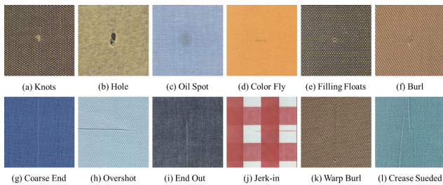
FIGURE 4. Common types of fabric defects.
