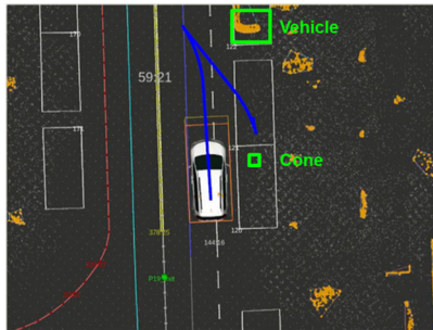
FIGURE 35. Common Parallel Back-left Trial 1 with the planning parking path.
