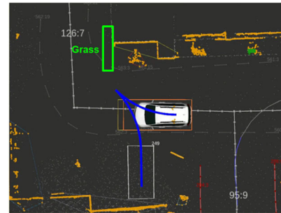
FIGURE 26. Common perpendicular left trial 1 with the planning parking path.
