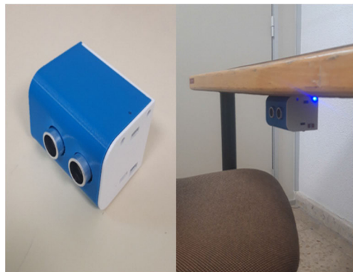
FIGURE 12. Assembly of the intelligent thing and its positioning in the inferior part of the desk.
