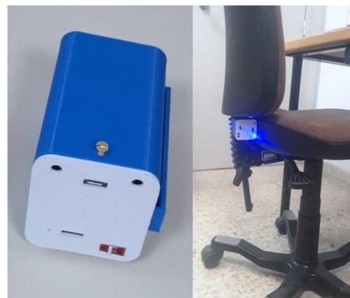
FIGURE 9. Assembly of the intelligent thing and its positioning in the inferior part of the chair.
