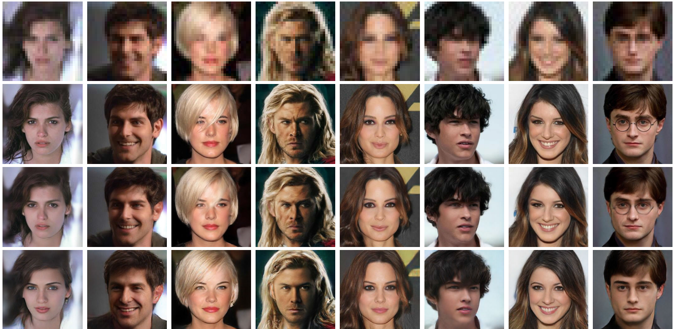
FIGURE 9. Comparison results when adding noise. Images from top to bottom: Input (Bicubic), GT, Ours (wo/ N), and Ours (w/ N). The upscale factor is 8x, the resolution of the input is 32 × 32, and the output is 256 × 256.
