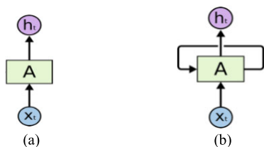
FIGURE 4. (a) The structure of a feed-forward neural network (b) the structure of RNN.
