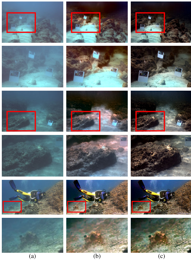
FIGURE 9. Effect of FSC. (a) Input images. The restoration results of the proposed algorithm (b) without FSC and (c) with FSC, respectively.
