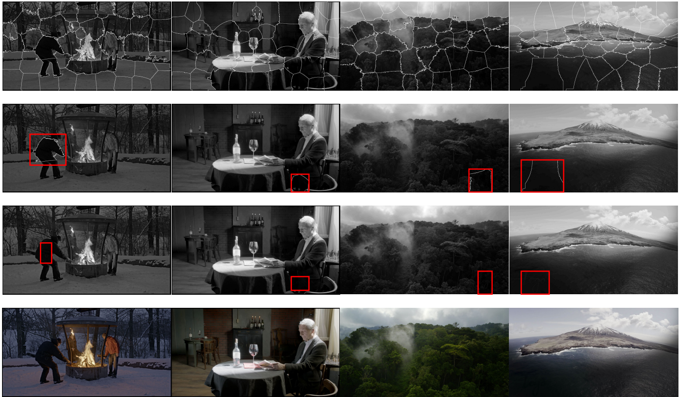
FIGURE 10. (1 st row) Superpixel segmentation on the Y-channel of various sample HDR images. (2 nd row) Corresponding target superpixel. (3 rd row) ER used to embed the watermark. (4 th row) Watermarked images after adding the color channels in 4:2:0 YUV format.
