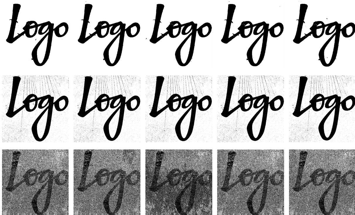
FIGURE 20. Binary watermarks extracted from BF_000 (Rec.2020 + PQ OETF) after applying various TMOs. (Left to right) TMO: C-TM, G-TM, H-TM, M-TM, R-TM. First row: proposed HDR-IW method. Second row: method in [8]. Third row: method in [9].
