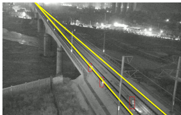
FIGURE 1. The detection of objects intruding into railway. Inside the yellow triangle is the alarm region. The objects in red bounding box are located inside alarm region and regarded as intrusions.
