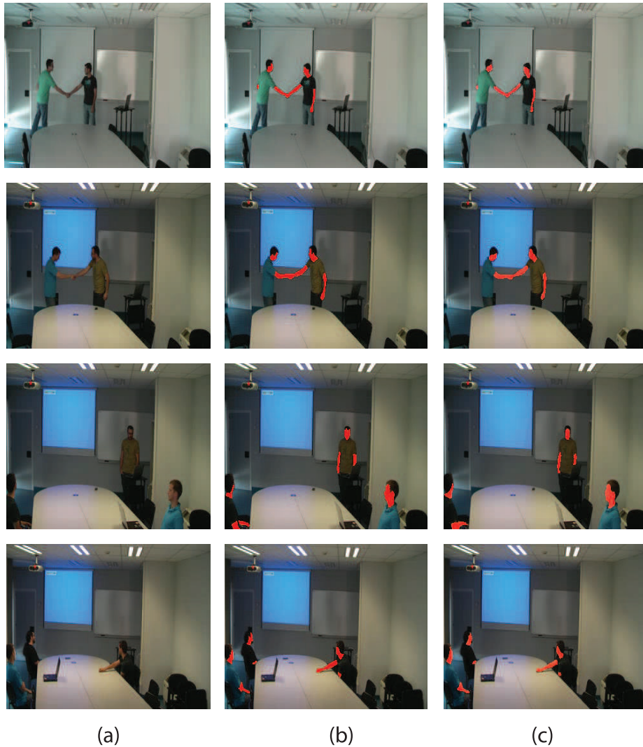
FIGURE 4. Example Images of EdDs datasets by SSS-Net that produces good segmentation results. (a) Image (b) Ground truth (c) prediction by SSS-Net. Red color presents the segmented skin area.
