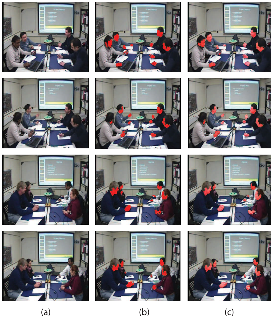
FIGURE 2. Example Images of AMI datasets by SSS-Net that produces good segmentation results. (a) Image (b) Ground truth (c) prediction by SSS-Net. Red color presents the segmented skin area.
