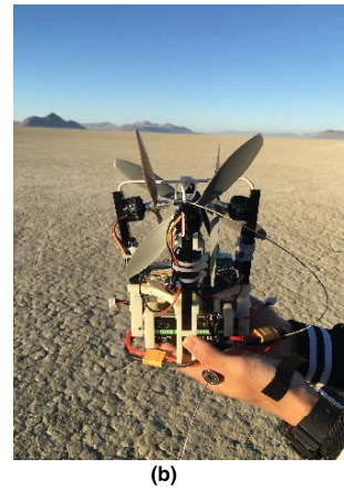
FIGURE 3. Foldable structure and inserted view of the foldable quadcopter. (a) Unfolded view of the foldable quadcopter. (b) Foldable view of the foldable quadcopter. (c) Inserted view in the airdrop container.
