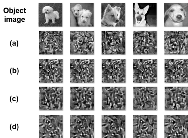
FIGURE 14. Retrieved images with the incorrect keys in the decryption process: (a) when the principal key p_2(x_0, y_0) is incorrect; (b) when the measurement matrix is incorrect; (c) when \lambda has relative error 3%; and (d) when d_1 has relative error 1%.
