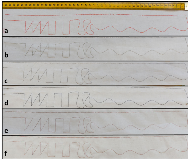
FIGURE 4. Embroidery performance of the different yarns, a) Ordinary embroidery yarn, b) Madeira, c) Shieldex, d) Tibtech as a bobbin yarn, e) Yarn A, and f) Yarn B.
