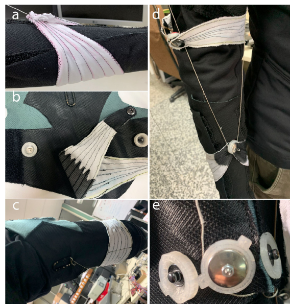
FIGURE 5. Textiles used to interact with the user. The stitches coincide with the force direction of the pulling cable; thus, transfer forces to the Anterior part of the limb. B shows the layers of the shoulder armband and clamp, including the inner reinforcement patches; the metal ring over the Triceps where to the elbow cable anchors is in c. The elbow cable, fixed to that metal ring, passes through the button-bearing in the elbow clamp balancing the pulling force, like shown in d. The elbow's pivot is in e, where the nylon coverage of the cable can also be seen. The pivot can be buttoned to three different positions what favours adaption to different arms' thicknesses.
