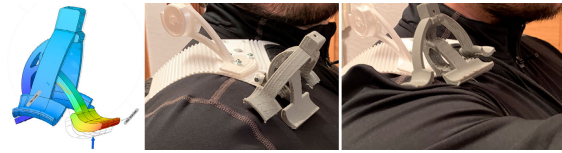
FIGURE 6. This piece acts as a pivot for the shoulder flexion. The base and deformation favours adaption during motion and distributes forces over the Pectoral. It is fixed to the wide base whose grooves favour fitting to the Trapezius. The left picture shows the deformation, in Autodesk Fusion 360, when a force of 90N is applied in the direction marked by the arrow. Maximum and minimum displacement is coloured from red to blue, respectively. The central and right images show the deformation and fitting of the piece when the shoulder performs a 90-degree flexion.
