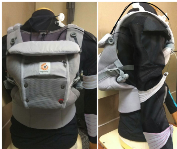
FIGURE 1. Exosuit to assist upper limbs flexion and backpack. This prototype uses an external power supply.
