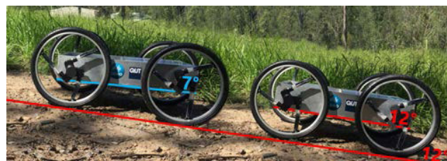
FIGURE 10. Experiments preformed on unstructured terrain in the field. Fig. shows unactuated wheels (right) and actuated wheels (left) holding the chasis level to the extremities of the wheel hub workspace. Terrain slope is 12 degrees.
