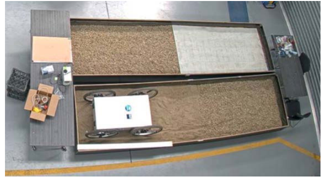
FIGURE 4. Two terrain boxes used for experiments, filled with sand and gravel. Rover is placed inside for scale.
