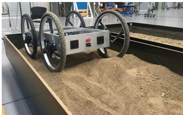
FIGURE 5. Rover in a terrain box filled with sand and gravel used for initial experiments with debuggng.
