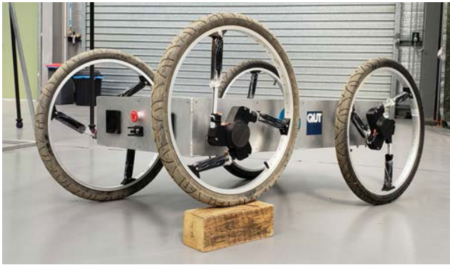
FIGURE 1. A rover utilising four Posable Hubs. The ride height of one wheel is manipulated to show its ability to climb an obstacle while maintaining a level chassis and ground contact with all four wheels.
