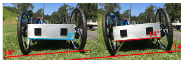
FIGURE 8. Fig. shown the rover on a sideways slope with unactuated wheels (right) and actuated wheels (left) holding the chasis level with gravity. The sideways slope has a gradient of 14 degrees.
