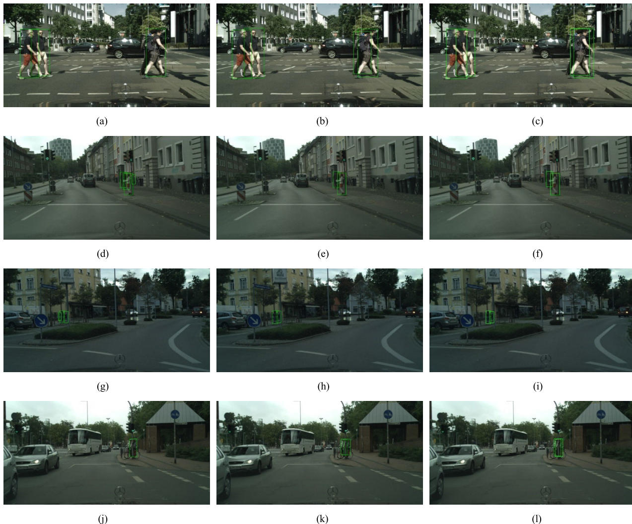
FIGURE 12. Visualization on CityPersons dataset. The images of each row from left to right are the detection results of FPN with 2 prediction layers, the detection results of our DA-Net, and the ground truths.
