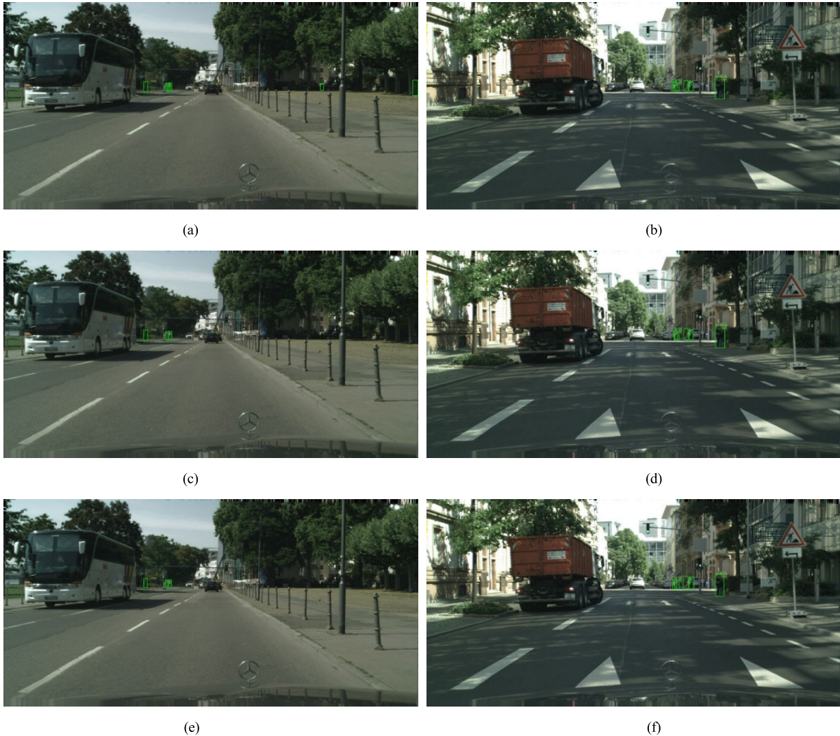
FIGURE 11. Comparisons between our network with DCB and without DCB on CityPersons dataset. The (a)(b) are the detection results of FPN with 2 prediction layers without DCB. The (c)(d) are the detection results of FPN with DCB. The (e)(f) are the ground truths.
