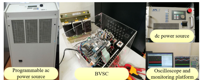
FIGURE 4. Experimental setup of fault-tolerant BVSC.
