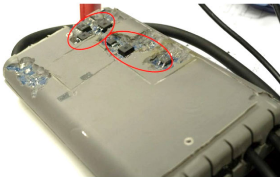
FIGURE 1. Photo of the disassembled PV microinverter with the thermally conducting epoxy removed at the locations of possible faults.
